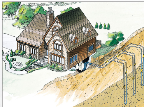
Example of a vertical, closed-loop system.
